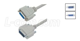
L-com's CHD26 family of hard to find high density D-sub cable assemblies offer solid performance at economical prices. Fully shielded throughout the entire cable to prevent against data corrupting EMI/RFI. Molded backshells provide superior strain relief while robust 26 AWG conductors are wired straight through for ease of compatibility. Metal thumbscrews insure fast and easy connections. Custom lengths and pinouts are available with modest minimum requirements.
